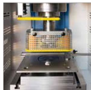
Punching tools set for diameters from 6 mm up to 160 mm
